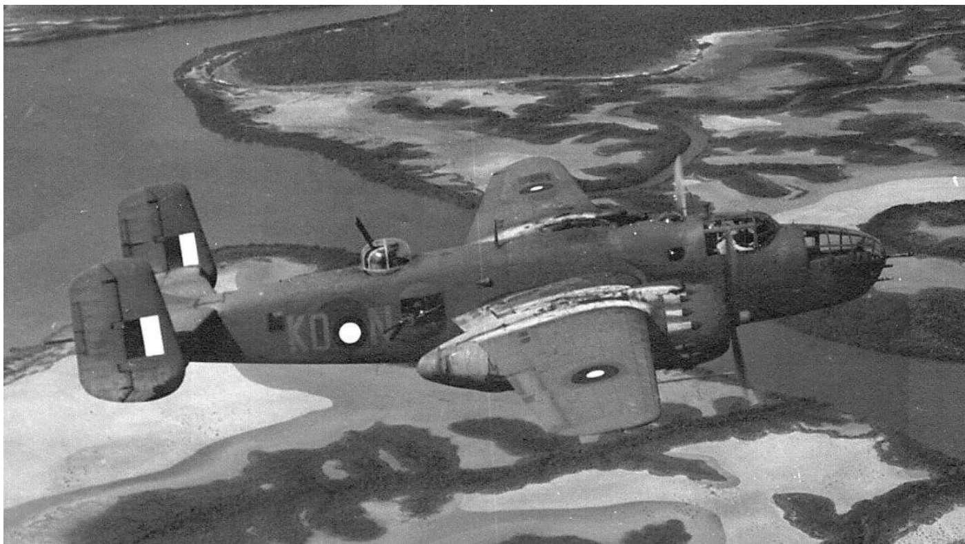
This is A47-5/KO-N, a non-Empty Shell Deflector B-25D-30-NC. It is seen here during 1944 displaying its factory applied OD41 over NG43 camouflage, 2AD applied Medium Sea Grey serial number (in deep shadow of the horizontal stabiliser) and 2SQN applied Medium Sea Grey code letters. [ adf-serials gallery ].
