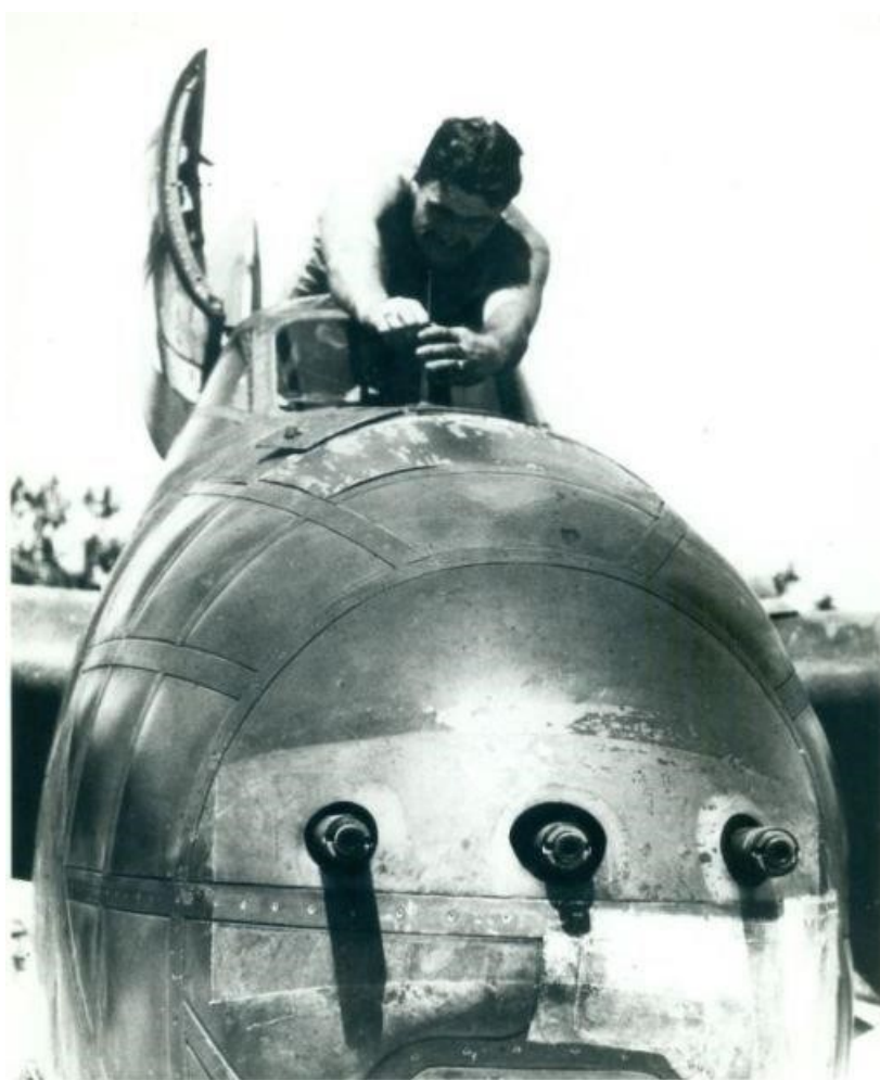
3 x .50 nose gun installation on RAAF A-20C, centre gun replacing AI radar antenna. [AWM OG 0374].
