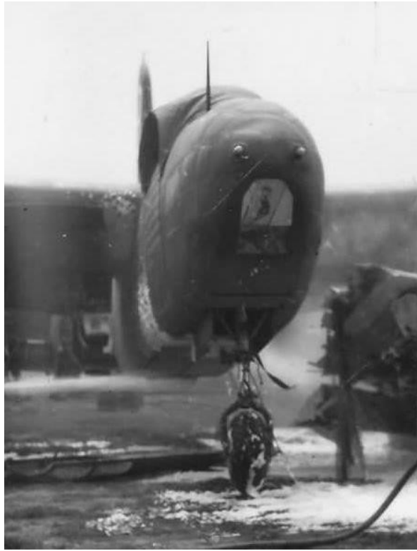
47 th BG USAAF North Africa A-20B with twin gun nose installation developed by Douglas and bomb aimers glass still retained. [47 th BG assoc.].
