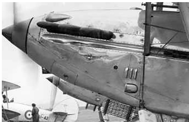
Different views of the “ram’s-horn” exhaust manifolds, with the 3SQN metal badge on the cowling
