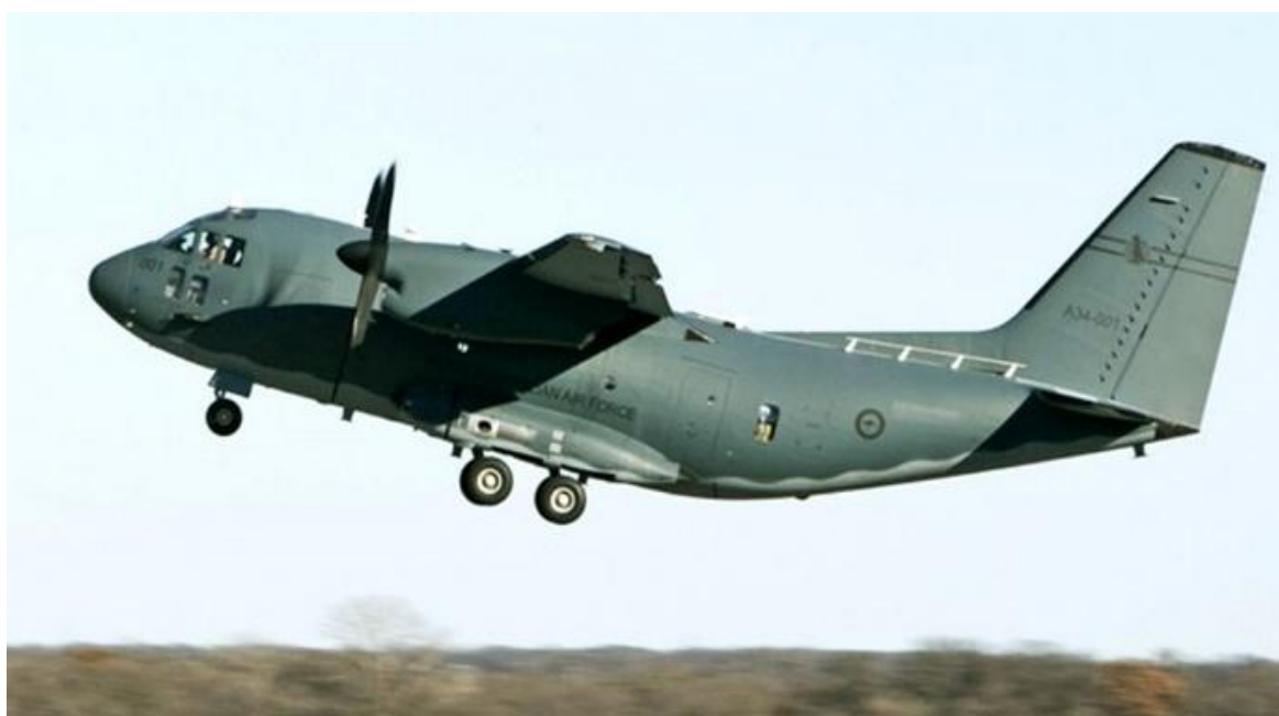
C-27J A34-001 Spartan provides a good example of toned-down markings – black roundel and no fin flash, black 35 Squadron marking across the tail, other detailing in black
