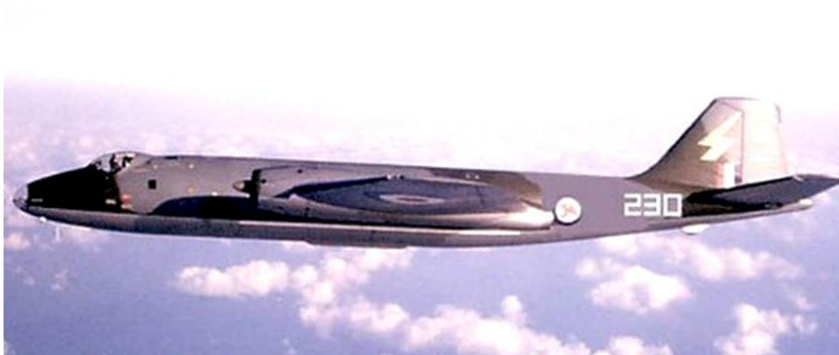
The first attempts at camouflage 1963-1964 – Canberra A84-230 of 1 Squadron, light grey/green upper surfaces, silver undersides with large main plane roundels, and large white serial numbers
