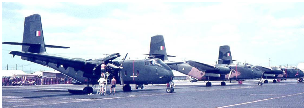
35 SQN Vung Tau, Vietnam 1970, shows A4-140 in gloss olive green overall (the original delivery scheme) and A4-159 in American camouflage (as the USAF serviced the Caribous in Thailand) – note fuselage roundels are reduced in diameter and there are no underwing national markings
