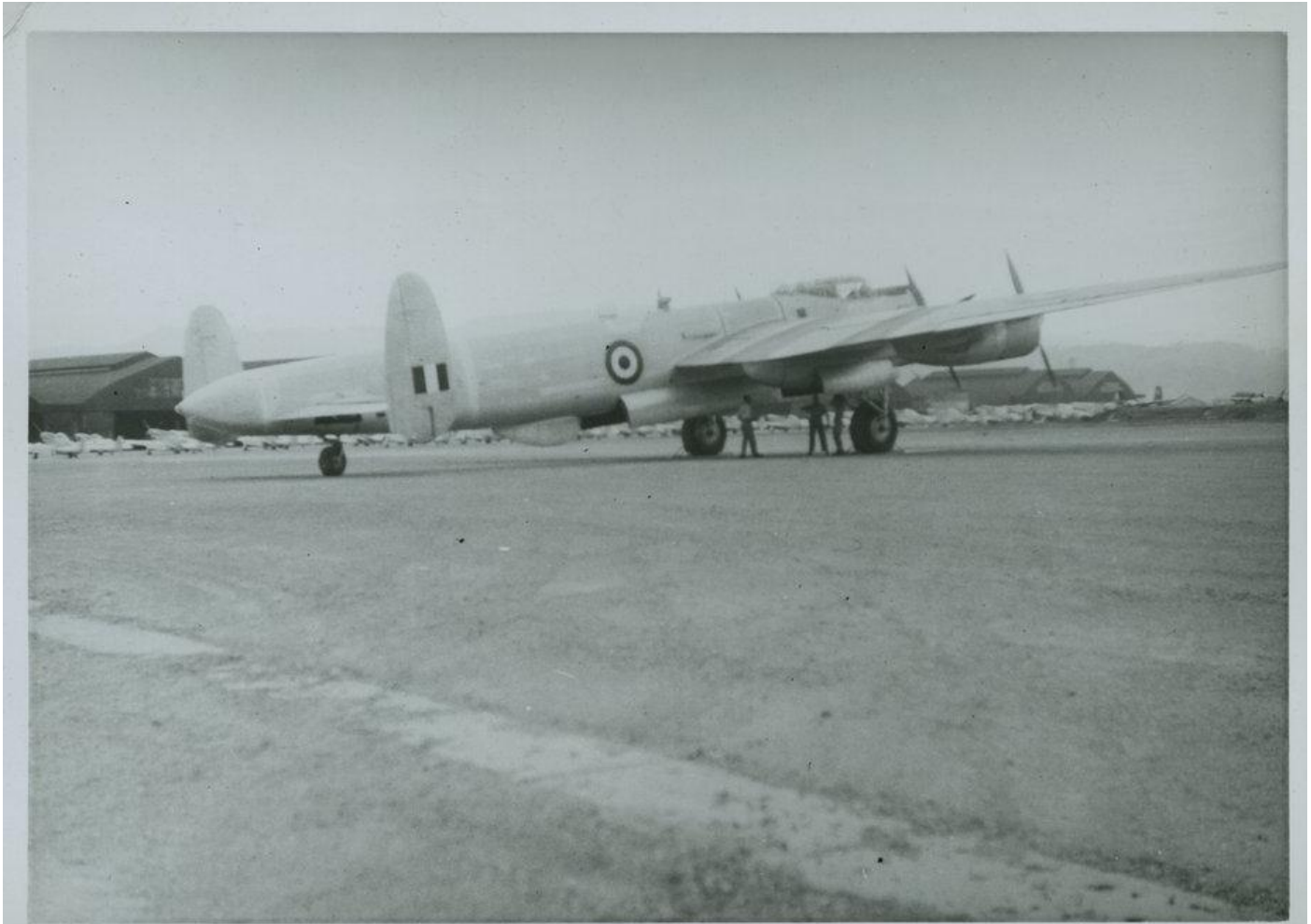
A73-2 Nyhuan in Japan 1948 with faired over Gun Turret positions and with DF Antenna
