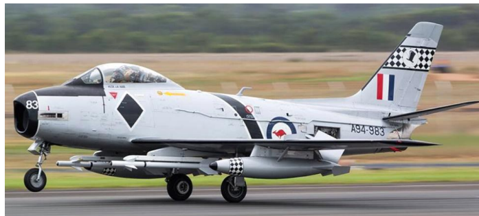
Early “Black Diamond” fin band A94-983 Mk.32 restored as a “Black Diamond” with small tanks
